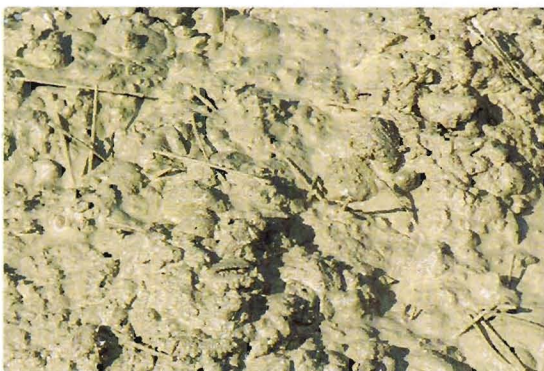
Figure 4 right: Barchip Macro is added at the concrete batching plant. Mix recommendations from EPC indicate Barchip should be added bag-and-all to initial water and prior to adding aggregate and cement.
